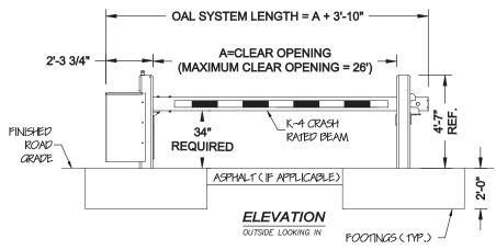
DENSITY OF NOT LESS THAN 95% MAXIMUM DRY DENSITY ARE REQUIRED. TYMETAL WILL NOT BE RESPONSIBLE FOR FAILED GATE OPERATIONS CAUSED BY UNSTABLE SOIL
