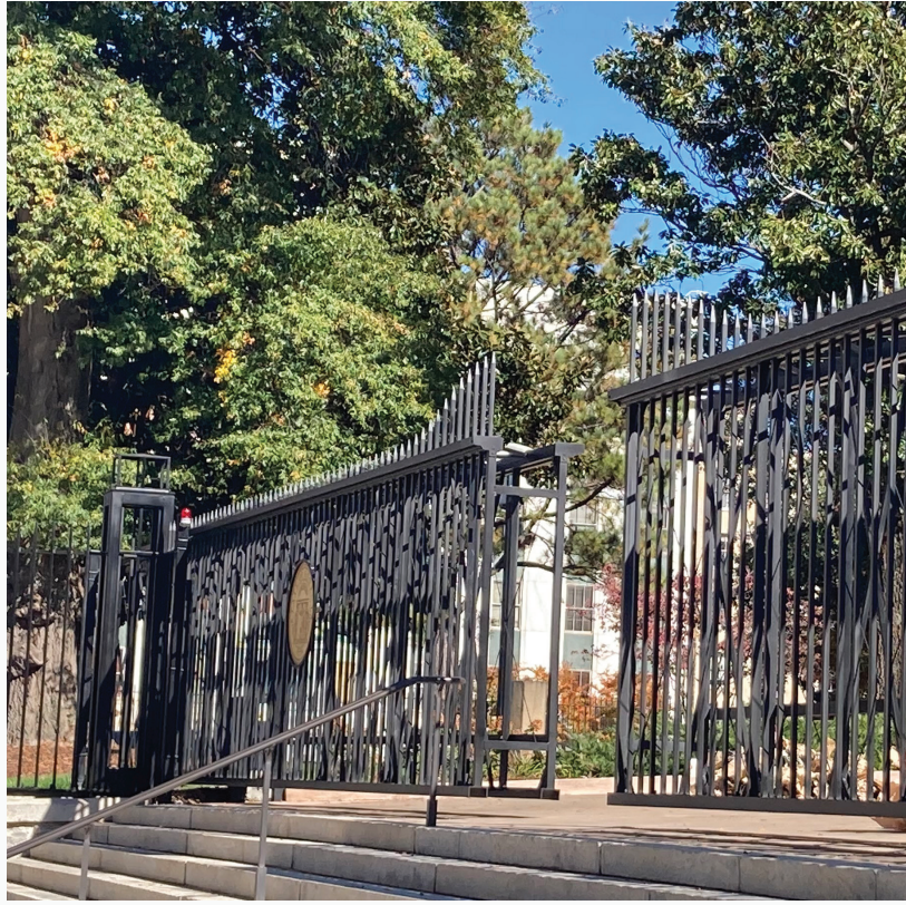
Right: Bi-Parting Box Frame Cantilever Gate with an opening of 61 feet. Pg. 15 for more details.
